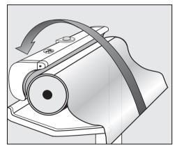
Hold the corners of the padding cover, pull taut and keeping taut lay over the heater plate.
