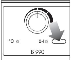
The rotary iron is turned on and off with the "**0-I**" button.
