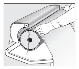
Insert the long edge of the new ironing cover into the retaining slot with the side seams inside (upside down). Keep side ties hanging free and smooth out.
