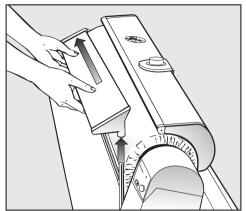
Lift the feed board out of the right hand holder and then pull it out to the left of the roller.
