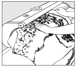
Fold in half with unironed edges together and place over the left end of the roller with the ironed middle section hanging over the edge to prevent creasing. Then pass both sides of the non ironed sections through the rotary iron.
