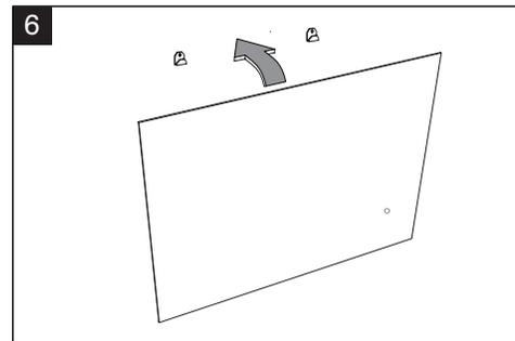
Install the mirror making sure the wall hangers are perfectly attached to the mirror back frame channel
