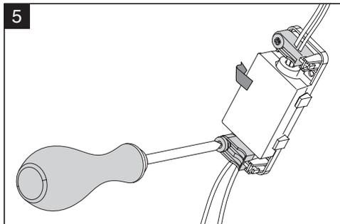
Close the clamp and fix it as shown in the drawing
