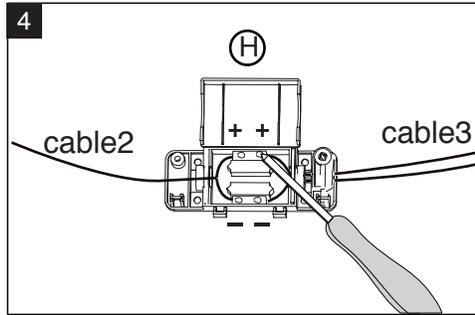
Connect clamp (H) with cable (2) of transformer (G) and cable (3) of the household power
