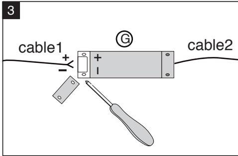
Connect cable (1) from the capacitive switch to the transformer (G) paying attention to the + and - signs of the two poles
